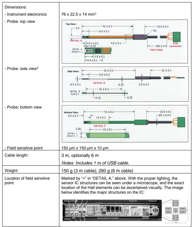
$<sup>^4</sup>$  The drawing shows probe version D0. Probe version D1 differs from D0 in that the thickness is 0.5 mm along the full 42 mm length, rather than 0.5 mm, 0.15 mm and 0.25 mm. Also see footnotes 2 and 3.
